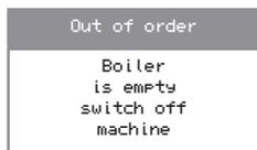
5. The software now knows the water system is empty. If the unit is reinstalled the commissioning menu will automatically be activated.
