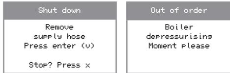
3. There is now no pressure in the boiler. The shut down menu can be cancelled if necessary. Follow the menu to empty the complete water system.
